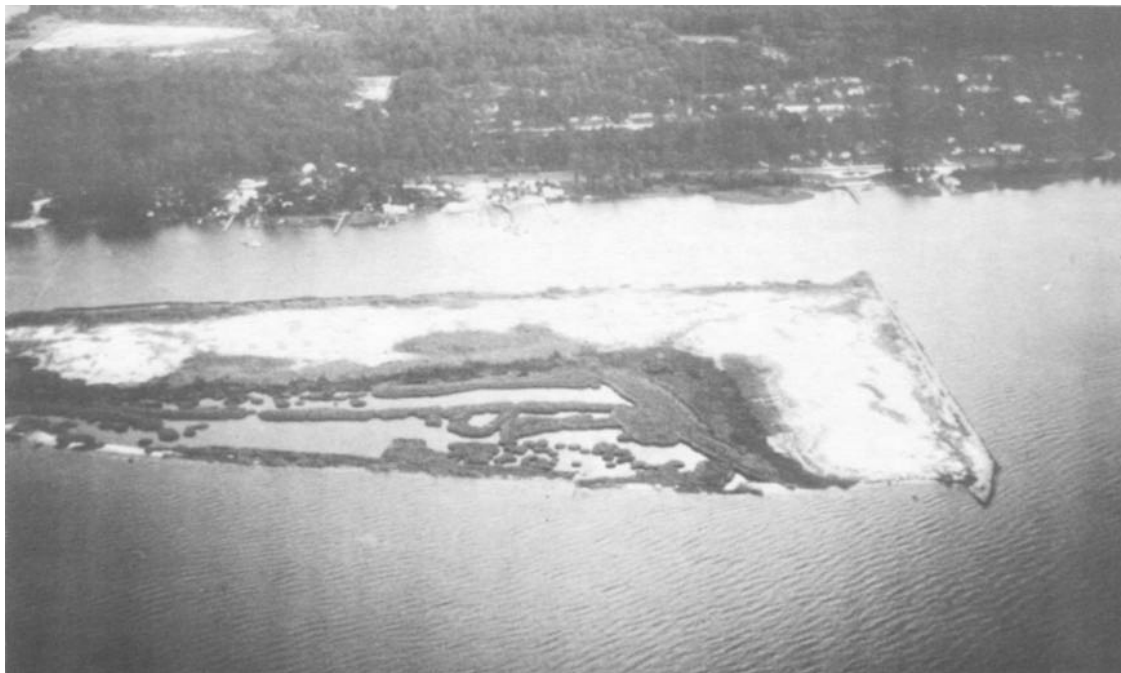
a. A salt marsh was established on poorly consolidated fine-textured dredged material confined behind an earthen dike on this dredged material island.
