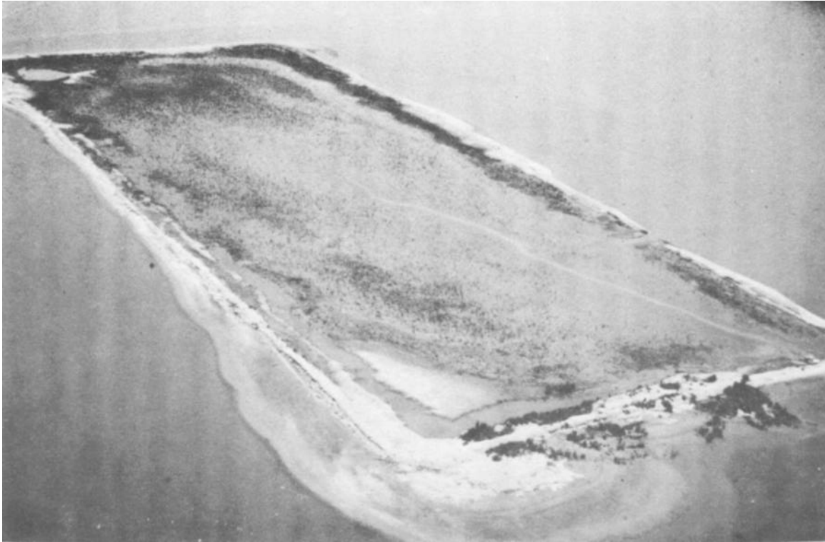
a. An aerial view of the 420-sq-ft freshwater marsh developed on fine-textured dredged material confined by a sand dike.
