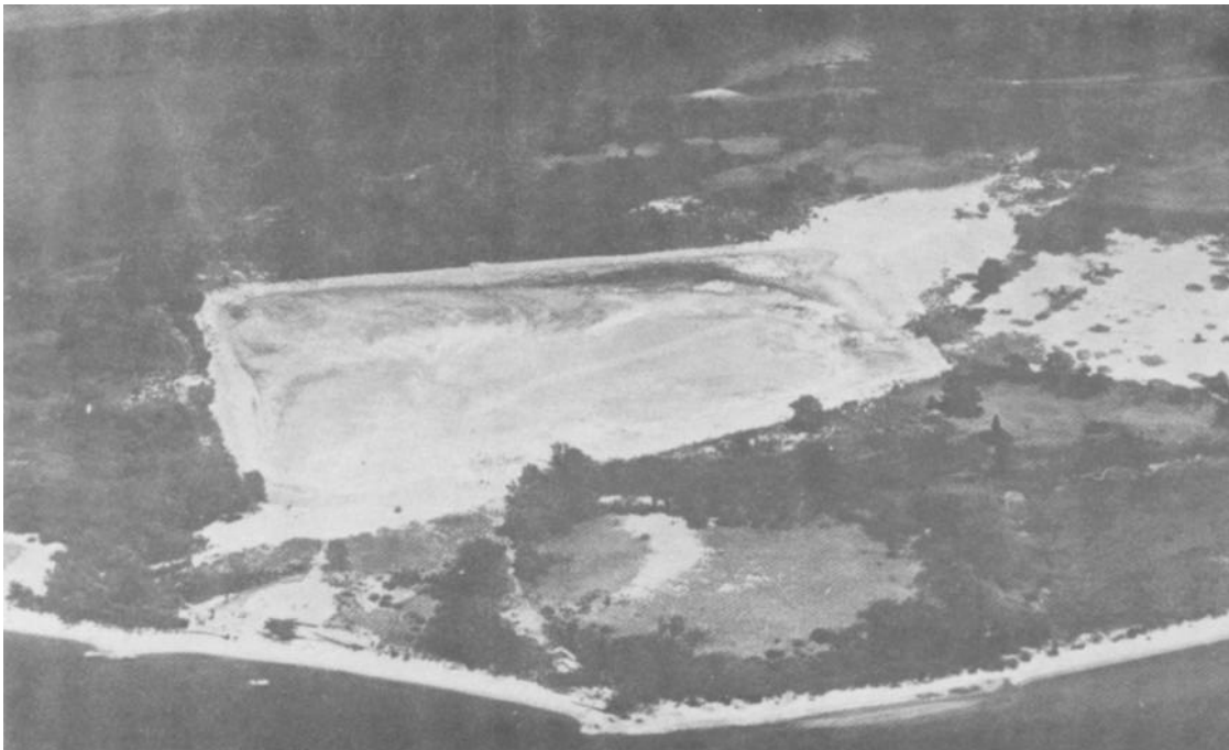
Figure 4-12. Sandy and silty dredged material were combined at Nott Island, Connecticut, to produce a pasture for wild geese.
